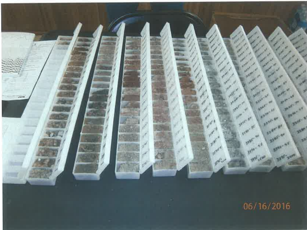
Drill cuttings down to 4,000 feet
